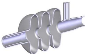
Figure 6 : Preliminary design of two couplers: a vertical coaxial line as main coupler and a beam pipe insert as LOM damper.
