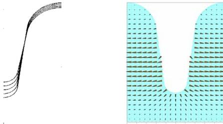
Figure 2 : MAFIA 2D model for cavity geometry design. Left: cavities with different irises. Right: typical electric field distribution of the deflecting mode.
