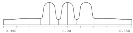
Figure 3: MAFIA 2D model of the 3-cell cavity design without couplers. The end cells are shorter than the central one and beam pipes at both ends are enlarged for couplers.
