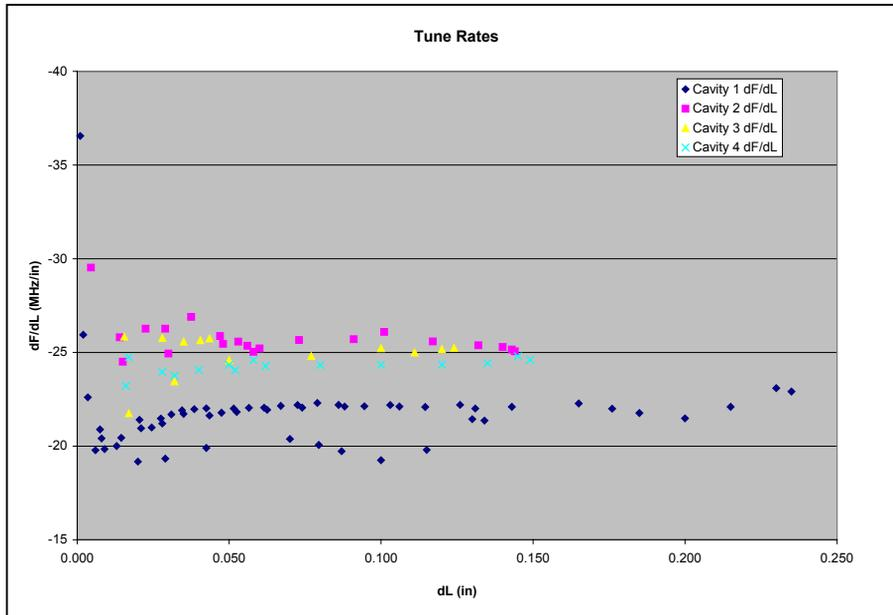
Figure 2, Cavity tune rates vs tune displacement
