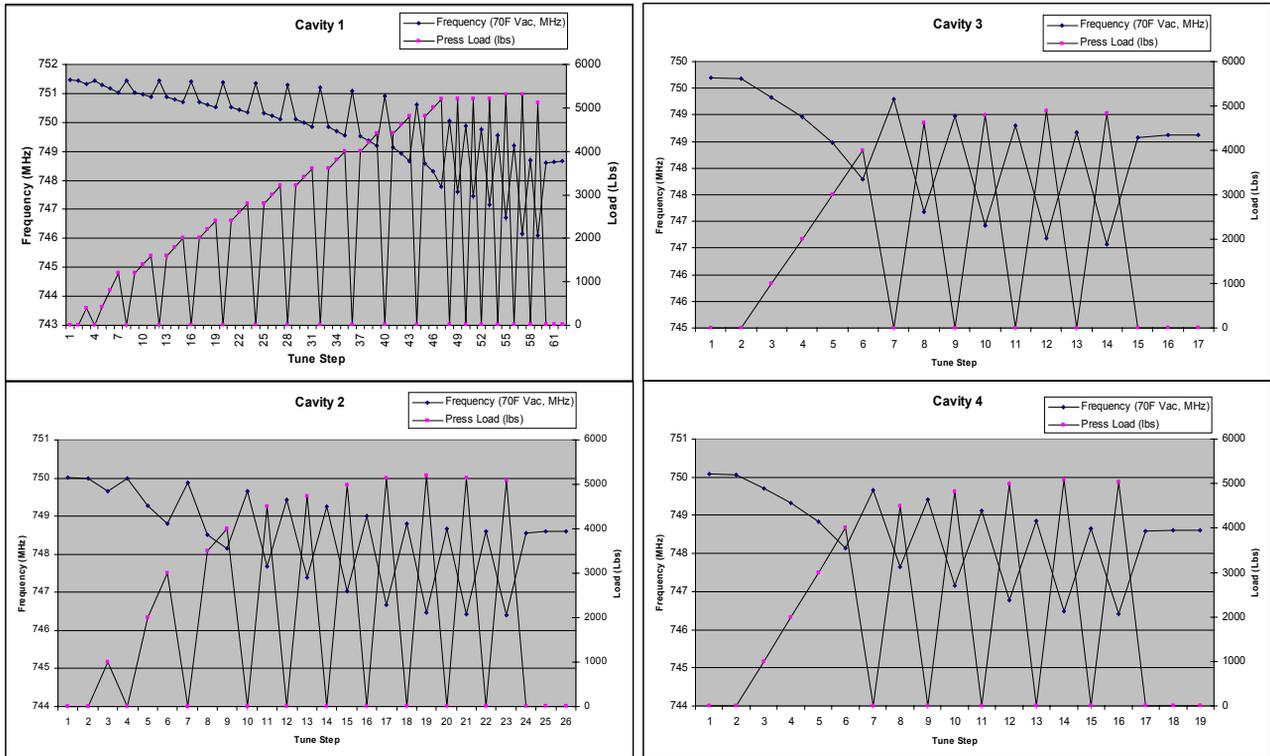
Figure 1, Cavity frequency and load during tuning
