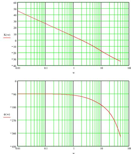
Figure 6. Slow tuner system open loop Bode plot for the stable operating region.
