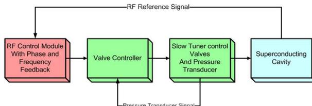
Figure 1: Block Diagram of the slow tuner system.
