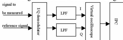
Figure1: The structure of the PAD.
