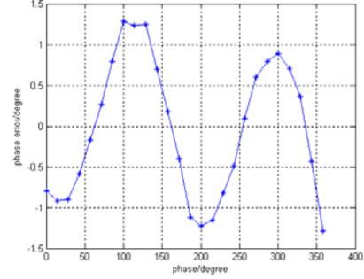
Figure 4: Phase error of the PAD
