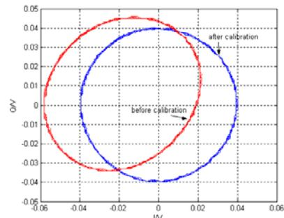
Figure 3: The I/Q trace before and after calibration.
