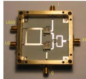
Figure 2: The I/Q demodulator.
