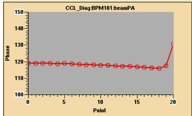
Figure 6: Beam phase vs. time with Adaptive FeedForward enabled. The variation in beam phase is reduced by a factor of ~20 compared to Figure 5. Beam parameters are unchanged.
