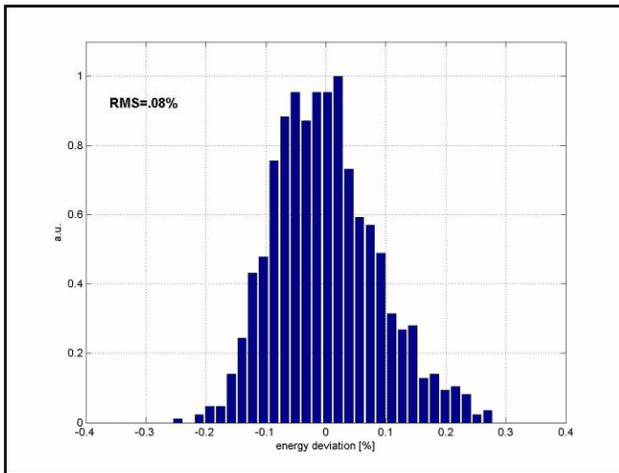
Figure 4: Beam energy spread measured downstream of DTL2 during April 2004 DTL beam commissioning. (courtesy of A. Aleksandrov).
