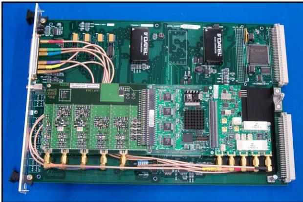
Figure 2: The Field Control Module is assembled and tested at SNS prior to installation in the Linac. The AFE, DFE and RFO daughter-boards are clearly visible from left to right.
