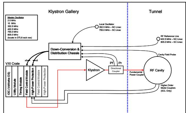
Figure 1: Block diagram of the SNS Linac LLRF control system.
