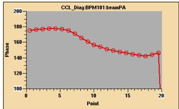
Figure 5: Beam phase vs. time at the entrance to CCL1 with Adaptive FeedForward disabled. Beam current is 40 mA. Beam pulse length is 40 us.
