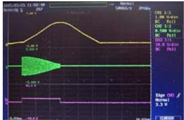
Figure 11: Waveforms of exciting current of bending magnet (CH1), gap voltage (CH2), and gate signal of rf system (CH3). (Time: 2ms/div.)
