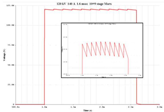
Figure 3. Staggered module switching to compensate for capacitor droop during the pulse.
