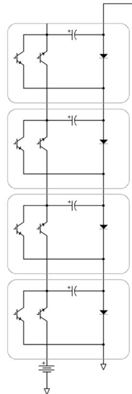
Figure 2. Four Stage Solid State Marx Bank Modulator (with switched recharge).
