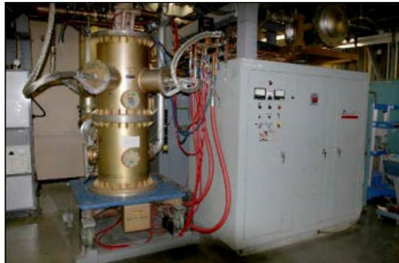
Figure 1: 201 MHz cavity amplifier and filament supply for the Burl 7835 triode.
