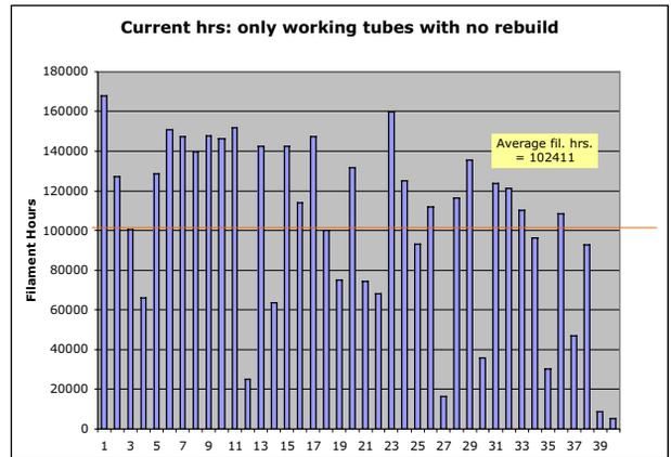
Figure 3: Total hours of all working klystrons that have not been rebuilt.
