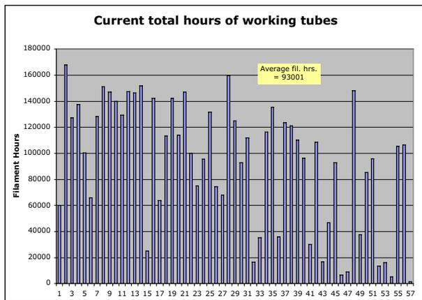
Figure 2: Total hours for all working klystrons.
