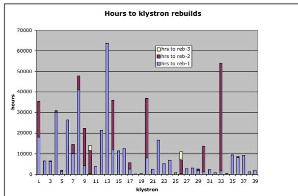
Figure 5: Hours to rebuild of all 39 klystrons that have been rebuilt, showing the hours to rebuild1, then rebuild 2 (in 18 cases), and then rebuild 3 (in 4 cases).
