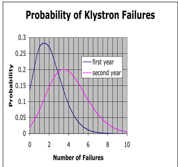
Figure 4: Probability of failure of currently operational klystrons in the first and second year.
