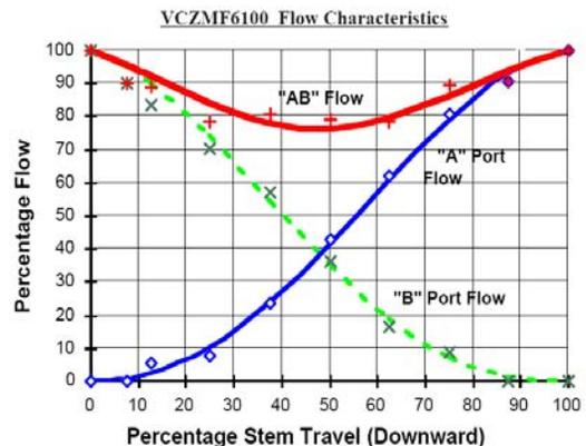
Figure 2: Typical 6100 series flow characteristics. [3]
