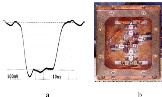
Figure 8: a-experimental waveform of 400 V 30 ns wide output pulse; b- 1250 W 125 Ohm RF load.
