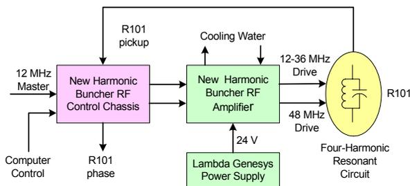
Figure 1: Four-harmonic buncher system block diagram.
