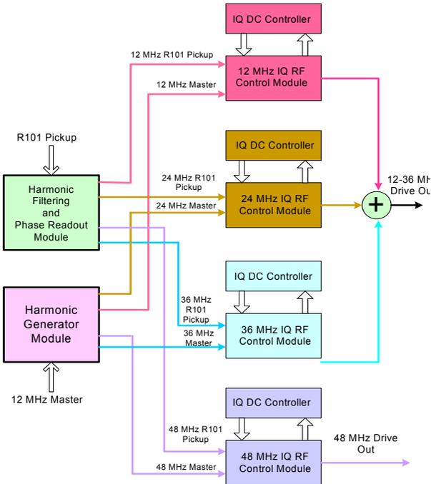
Figure 3: I & Q RF controller block diagram.
