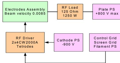
Figure 5: TWC system block diagram.
