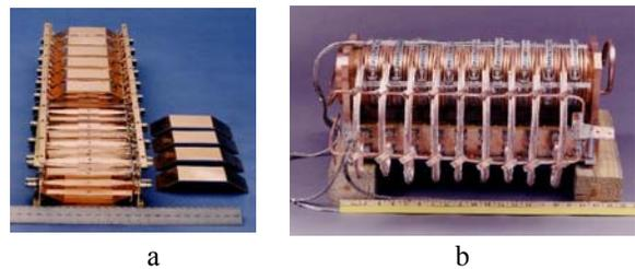
Figure 6: a-stripline deflection section, b-delay lines.
