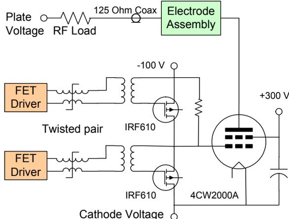
Figure 7: Simplified diagram of the RF driver. FET driver boards are DEI FPS-3N series fast power switch.
