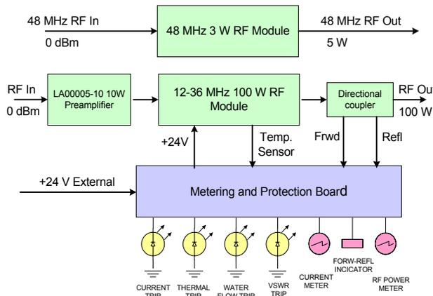
Figure 2: RF amplifier block diagram.
