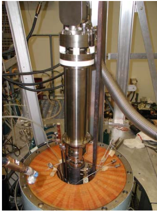
Figure 7: View of the new collector installed on the magnicon, prior to installation of the pole piece.
