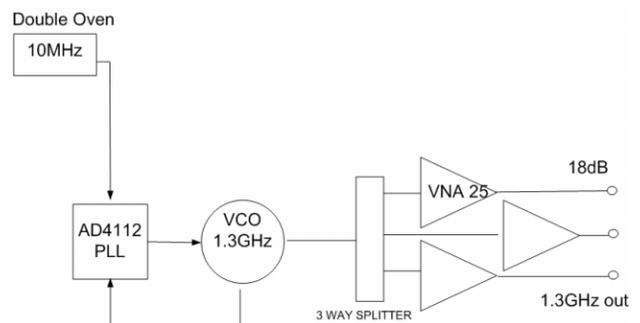
Figure 2: PLL and VCXO 1.3GHz Oscillator.
