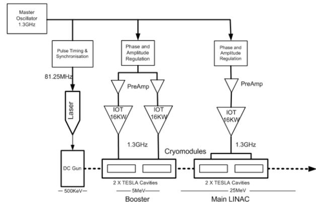
Figure 1: Basic RF system architecture.
