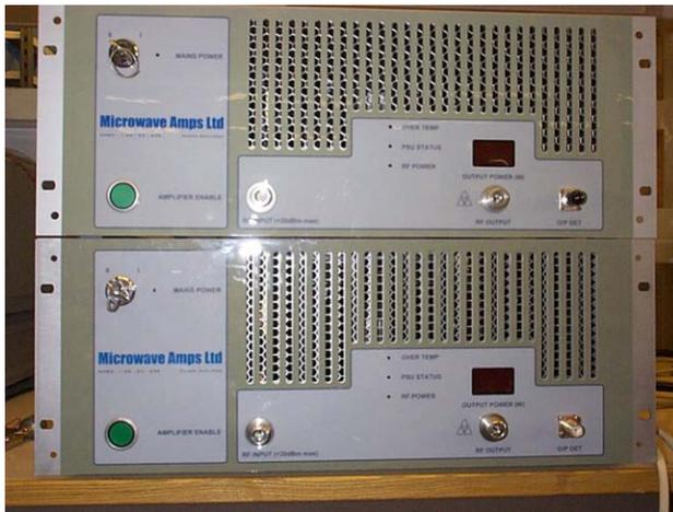
Figure 6: Microwave Amplifiers 1.3 GHz 250 W Amp.
