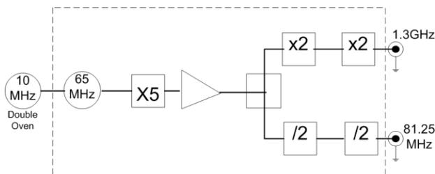
Figure 3: Multiplier based oscillator.
