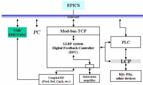
Figure 5: The basic interface configuration between the LLRF system and EPICS control system.
