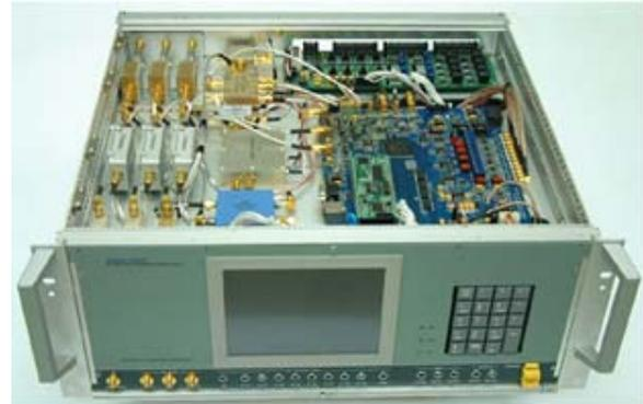
Figure 3: The photograph of the digital feedback RF control system.
