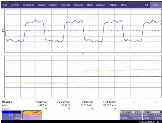
Figure 2: The characteristics of the PLL clock generator.
