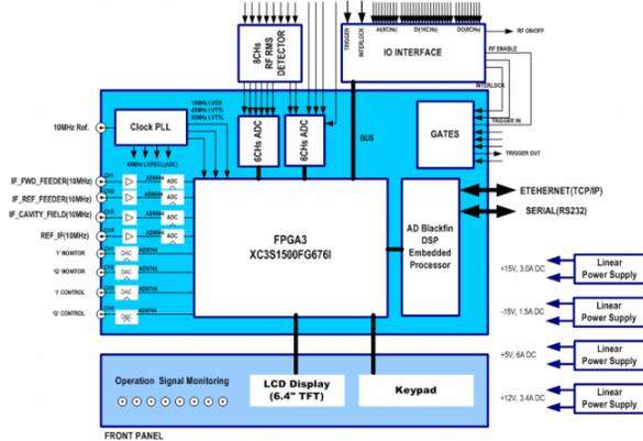
Figure 1: The detailed configuration of the digital feedback RF control system.
