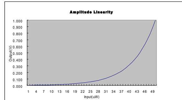
Figure 4: RF signal (350MHz Carrier) amplitude linearity of the digital feedback RF control board.
