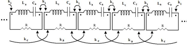
Figure 1: Circuit representation for a biperiodic chain of cavities with first ( $k_1$ ) and second nearest neighbor ( $k_{a,c}$ ).
