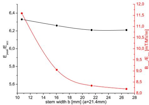
Figure 8: Electric and magnetic peak fields in dependence of the stem width a.
