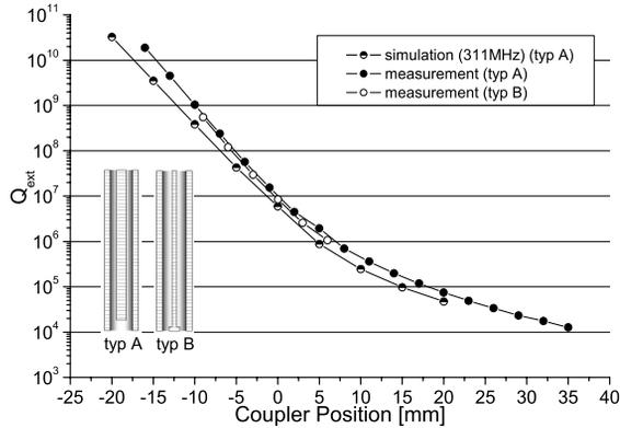
Figure 3: Calculations and measurements on capacitive couplers for the copper-model (Fig.2) of the CH-Cavity. 0mm corresponds to the girder surface plane.
