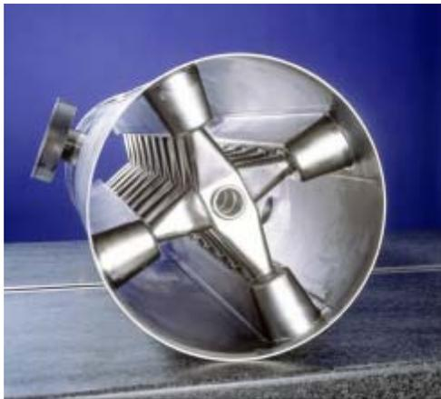
Figure 1: The sc 352 MHz CH prototype
