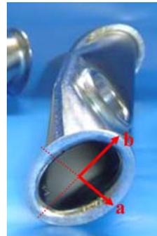
Figure 6: Stem of an sc CH-Cavity.
