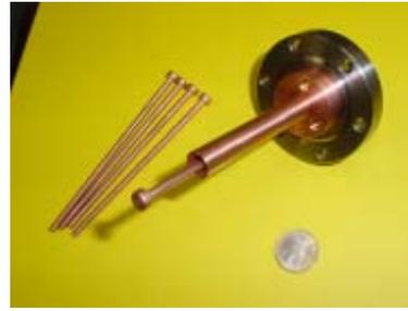
Figure 5: Coaxial coupler for the first cold tests.
