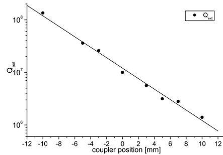
Figure 10: Qext for the optimized Cavity.
