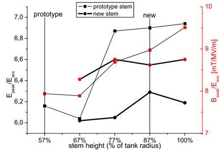
Figure 7: Electric and magnetic peak fields in dependence of the girder height
