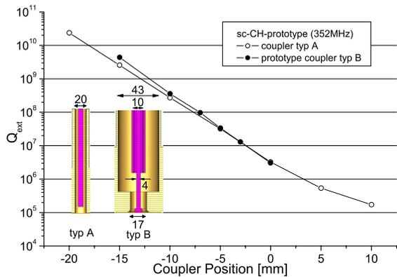
Figure 4: Calculations on capacitive couplers for the s.c. prototype of the CH-Cavity.
