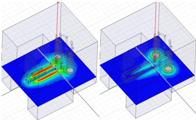
Figure 6: Magnetic and electric field distribution for simplified PA model at operating frequency of 23 MHz.
