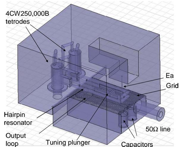
Figure 5: 3D HFSS model of output resonator for push-pull PA with 4CW250,000B tetrodes.
