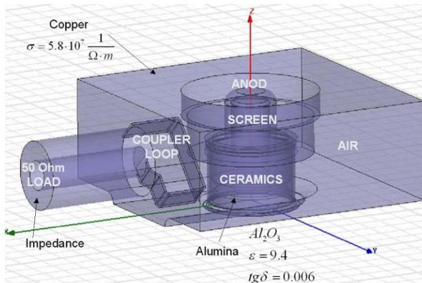
Figure 1: HFSS 3D model of the RF Booster Amplifier.
