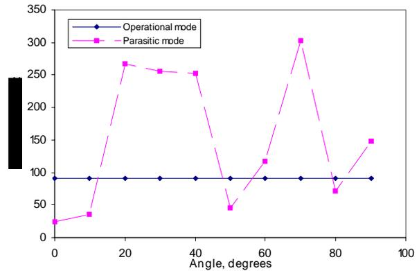
Figure 4: Nearest eigen mode's frequencies dependence on the coupler loop orientation.
