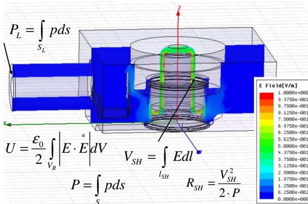
Figure 2: Operating mode electric field distribution in the amplifier output resonator.
