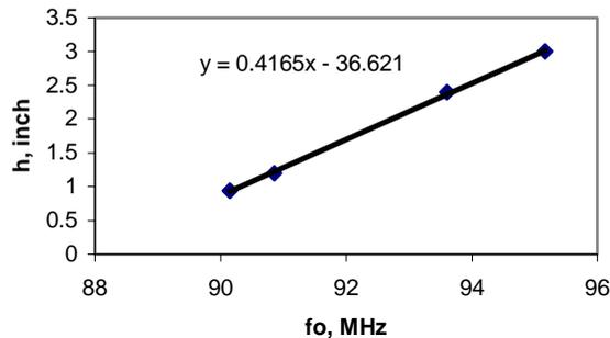
Figure 3: Fixed tuner adjustment curve for the modified output resonator.
