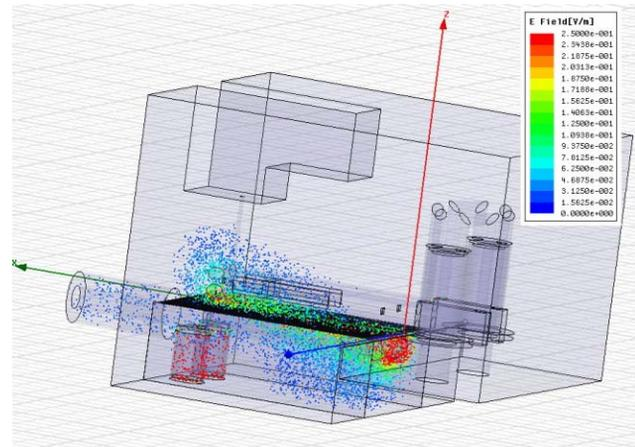
Figure 7. Magnetic field distribution in the cavity at operation frequency obtained from HFSS Eigensolver for full model.
