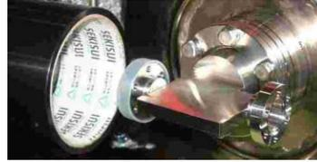
Figure 5a: Flat chamber for 180-degree bending magnet.
