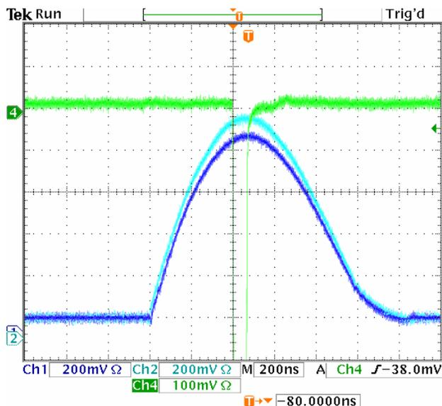
Figure 4: Trigger and the two kicker pulses.
