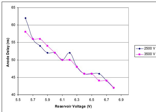
Figure 3: Anode delay time vs reservoir voltage.
