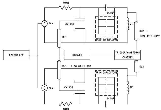
Figure 1: Schematic of the new PEP injection kicker system.
