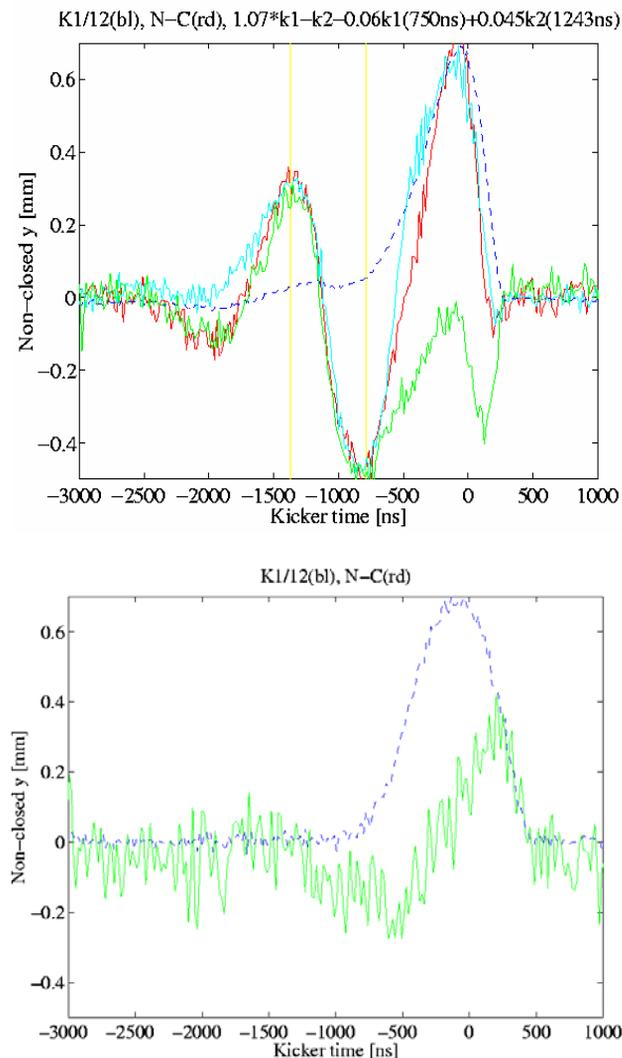
Figure 5: Old (top) and new (bottom) beam response due to injection kickers. The blue, dashed line is the main kick from kicker 1 (K1) divided by 12. The green is the closure of the two pulses.
