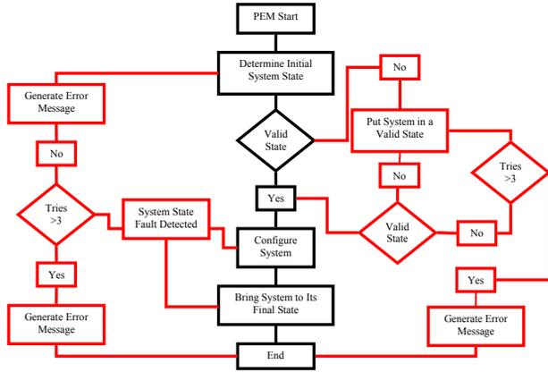
Figure 1: PEM machine procedure high-level flow diagram.
