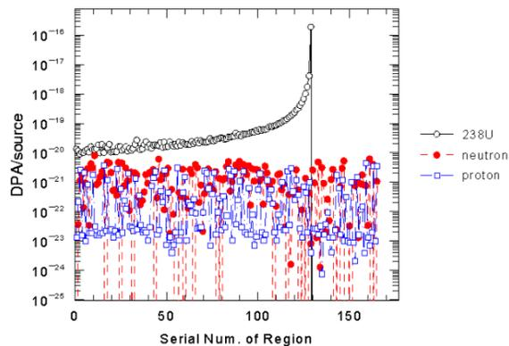
Figure 4: DPA from 320 MeV/A U ions on Cu beam dump as a function of depth, case of 1 μm-thick regions.
