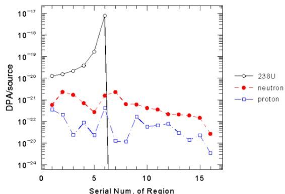
Figure 3: DPA from 320 MeV/A U ions on Cu beam dump as a function of depth, case of 25 μm-thick regions.
