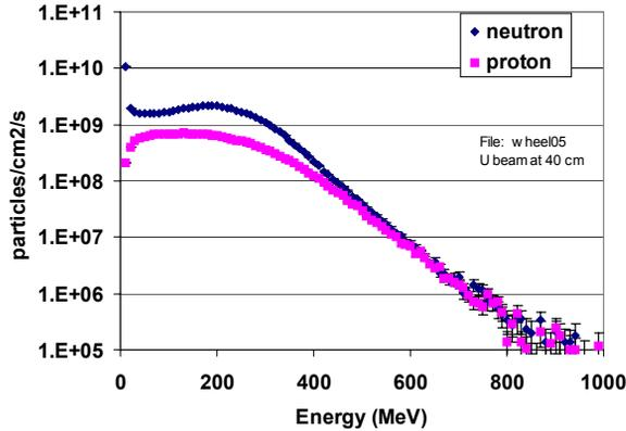
Figure 2: Neutron and proton flux in the wheel.
