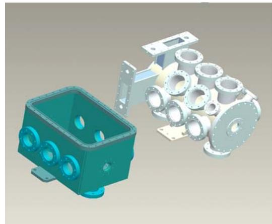
Figure 1: Anti-chopper and new diagnostics chamber.
