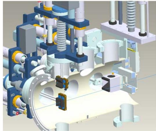
Figure 2: Emittance system and beam stop.
