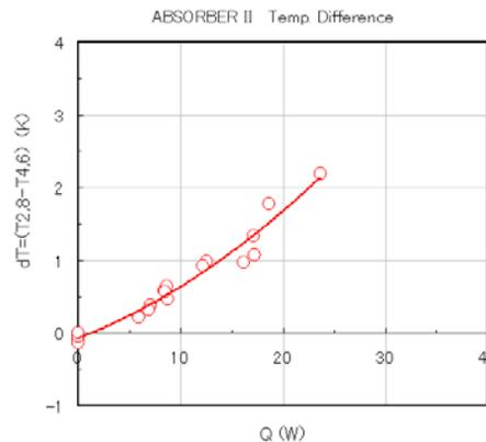
Figure 5: Maximum temperature difference in absorber vs. cooling power in the LH<sub>2</sub> absorber.
