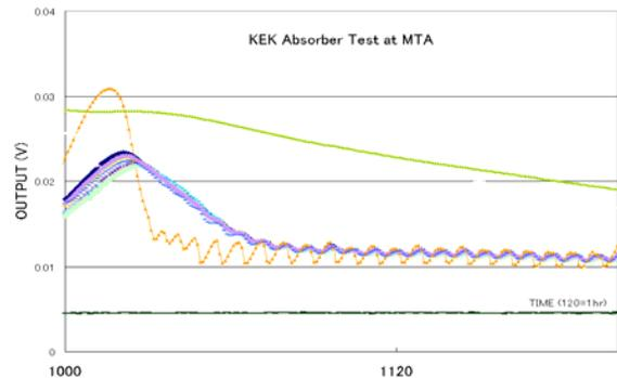
Figure 4: Thermal vibration at ~25 K (the vertical axis is the reading of thermometers in volts, the horizontal axis is the run time in seconds)
