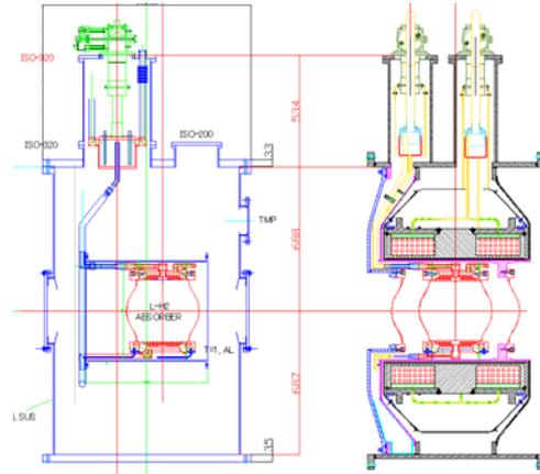
Figure 7: Plan views of the LH<sub>2</sub> absorber inside the AFC module cryostat with cryocooler (left) and within the focussing solenoid (right).
