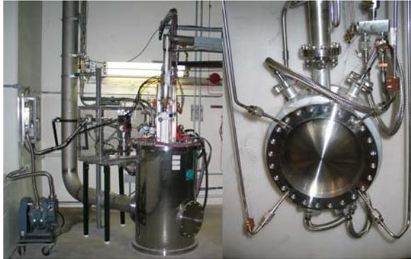
Figure 2: Setup for convection LH<sub>2</sub> absorber: Convection LH<sub>2</sub> absorber with He gas heating/cooling lines (right) and the cryostat at the MTA (left).
