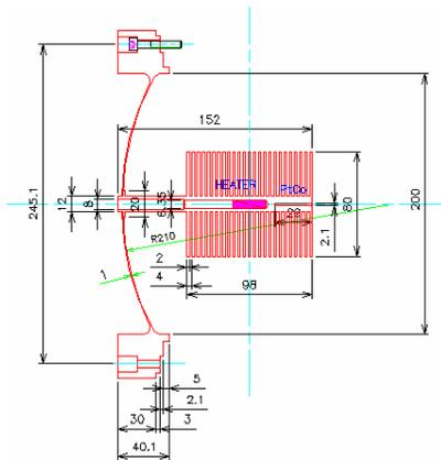
Figure 6: Plan of electrical heater and fins in the absorber (attached from the window).
