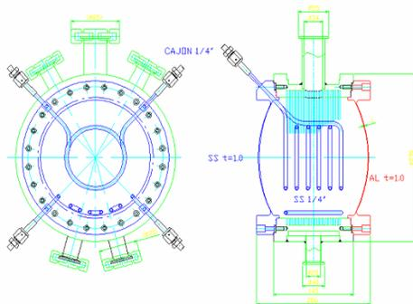
Figure 3: Cooling and heating He gas lines inside the LH<sub>2</sub> absorber.
