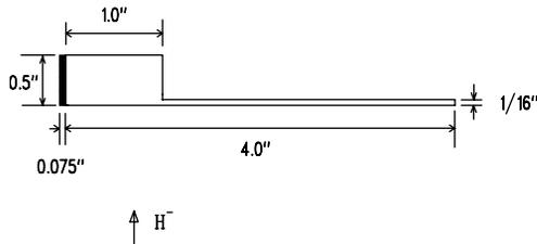
Figure 7: Plan view of the proposed step-shaped finger 5 and its thickness. The leading portion 0.075 inch represents fingers 1-4.
