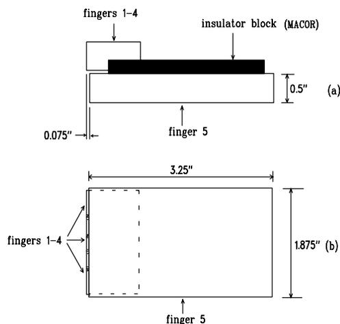
Figure 1: Schematic diagram showing the plan view (a) and front view (b) of LE2 fingers.
