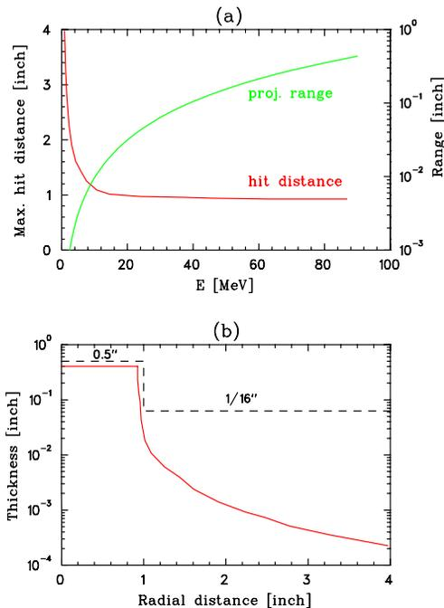
Figure 5: Max. hit distance and projected range in copper vs the energy of proton (a), and thickness of finger 5 vs the distance from the probe tip (b). The dash line suggests a step shape for easier machining.
