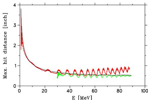
Figure 2: Calculated maximum hit distance of beam from the probe tip as a function of the energy. Red: result from starting at injection gap; Green: result from starting at 30 MeV with finite emittance and a displacement of 0.2 inch at start; Black: analytical result.
