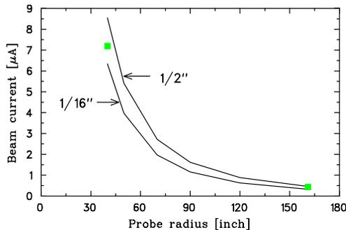
Figure 6: 1-D WAERME[3] calculated beam current to yield a maximum temperature of 350°C at several radii. The plate thickness was assumed to be uniform and either 1/16 or 0.5 inch; copper emissivity was 0.4. Filled squares: results from 3-D ALGOR calculations where the finger thickness used is a step-shape as is shown in Fig. 7.
