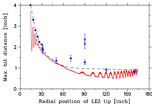
Figure 4: A comparison of the measured (filled squares: HC4 off; open squares: HC4 excited) and the simulated (solid line, from Fig. 2) results of the maximum hit distance vs LE2 tip radius. The dash line is a fit through the filled squares.
