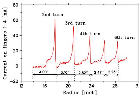
Figure 3: Measured differential (summation over fingers 1-4) scan of successive turns of beam using probe LE2.
