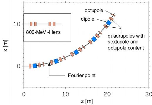
Figure 1: Layout of strawman five-cell 800-MeV proton achromat. The 800-MeV  $-I$  lens is shown for comparison.
