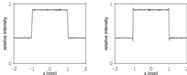
Figure 9: Intensity profiles of simple-object image, for 23-GeV BNL  $-I$  lenses configured as described in text.
