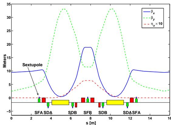
Figure 1: The above plot shows the location of the sextupoles in the lattice and the corresponding optical functions. In this case the optics has been configured for zero dispersion in the straight sections.
