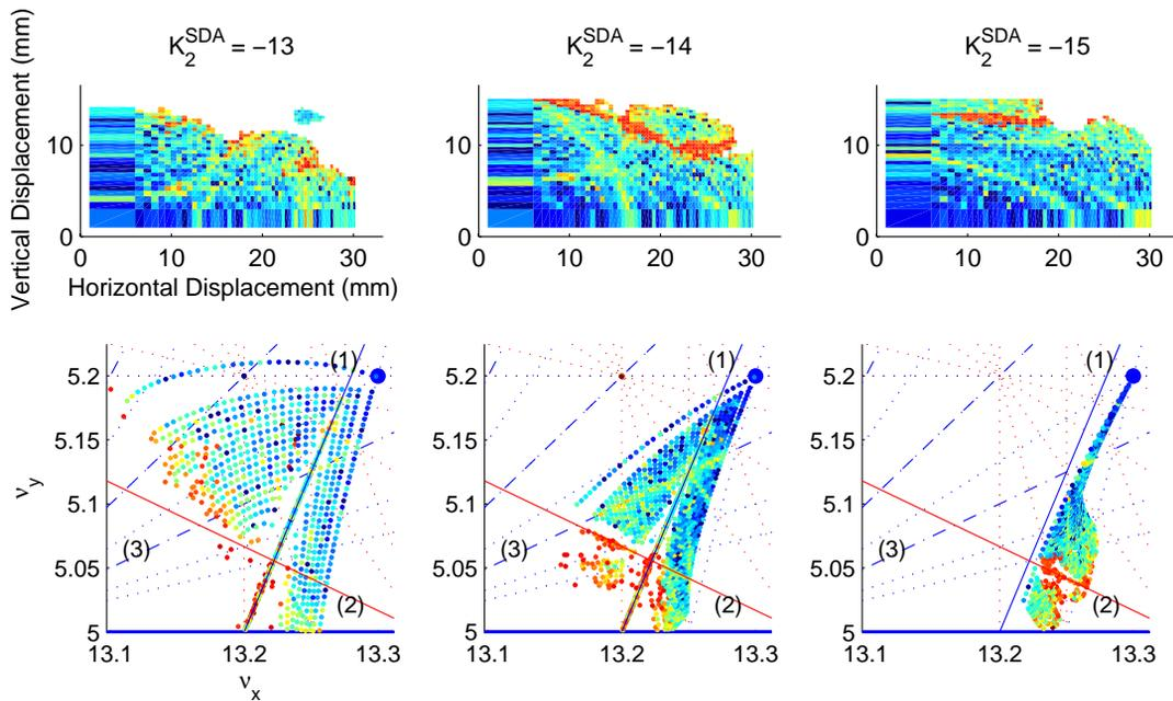
Figure 3: In the cases above  $k_2^{SFA} = 14$  and  $k_2^{SDA}$  was varied. The plotted lines show both sum (red) and difference (blue) resonances up to 5th order. The labelled resonances are (1)  $5\nu_x - 2\nu_y$ , (2)  $3\nu_x + 6\nu_y$  and (3)  $\nu_x - 2\nu_y$ . The vertical tunes shift with amplitude is along the side of the triangle closest to the label (1) and the horizontal tunes shift with amplitude along the side closest to (2).
