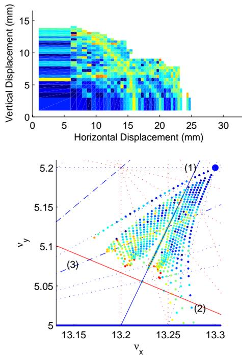
Figure 4: In the cases above  $k_2^{SFA} = 14$  and  $k_2^{SDA} = -14$  with the measured harmonics (allowed) of the quadrupoles. This should be compared to the centre plots in Figure 3.
