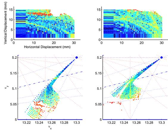
Figure 5: In the cases above  $k_2^{SFA} = 14$  and  $k_2^{SDA} = -15$ . The plots on the left do not have thin sextupoles while those on the right do.
