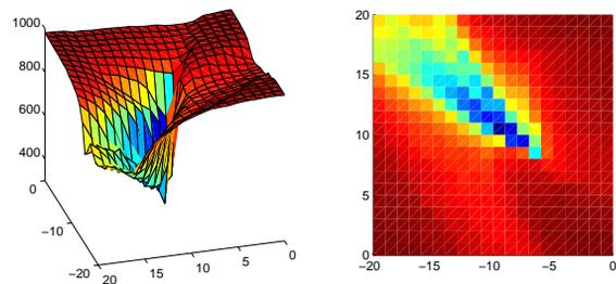
Figure 2: The above plot shows the number of particles that were lost at 1000 particles were tracked for 1000 turns. A global minimum is observed around  $k_2^{SFA} = 10$  and  $k_2^{SDA} = -10$ .
