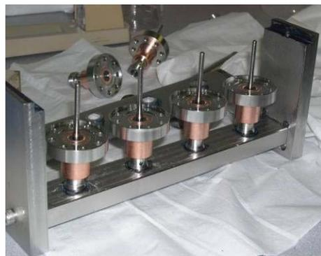
Figure 4. JLab single-crystal sapphire RF feedthroughs.
