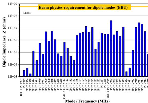
Figure 3. Impedance of dipole modes of 7-cell LL cavity LL003 with four HOM couplers in the JLab VTA. ( $Z = (R/Q)_T \times Q_0$ ).
