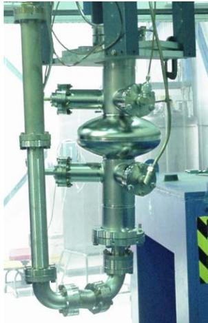
Figure 2: Single cell cavity used for the simultaneous excitation of the  $TM_{010}$  and  $TE_{011}$  mode.
