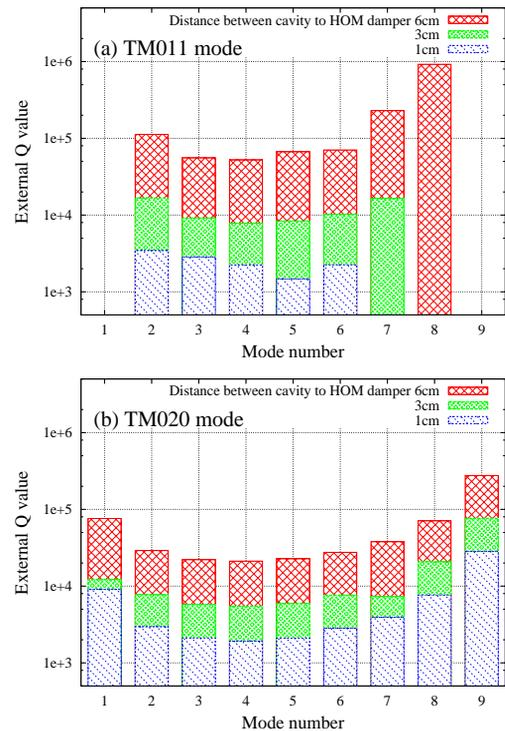
Figure 4: Measured  $Q_{ext}$  for the (a) TM011 and (b) TM020 modes. The red, green and blue bars indicate the results under the conditions of (2), (3), and (4), respectively.
