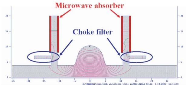
Figure 1: Conceptual design of the radial-line HOM damper.
