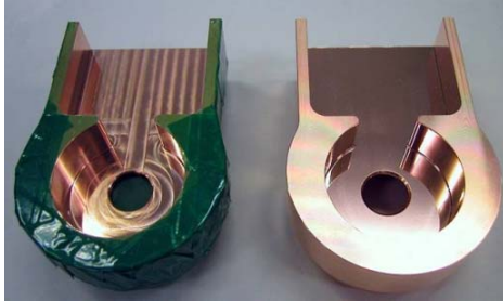
Figure 5: Effect of electro-polishing: Left and right coupler bodies are before and after electro-polishing, respectively. The cutter marks are disappeared by polishing.
