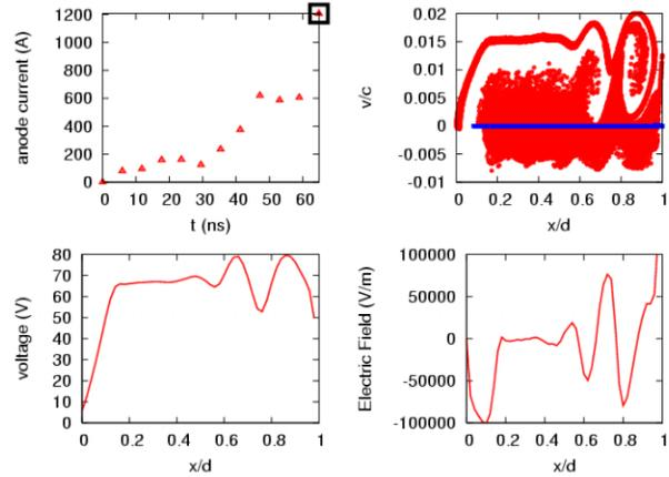
Figure 3: The phase space (upper right), voltage (lower left), and electric field (lower right) at 65ns after the start of electron flow. Ions are shown in blue. For reference, we also show the time history of the anode current (upper left), with the relevant time indicated with a square.
