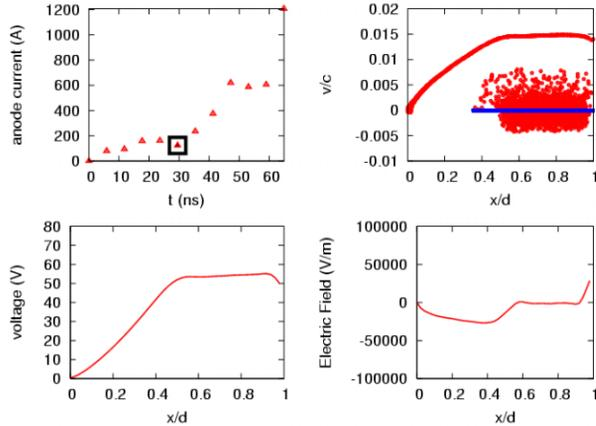
Figure 2: The phase space (upper right), voltage (lower left), and electric field (lower right) at 30ns after the start of electron flow. Ions are shown in blue. For reference, we also show the time history of the anode current (upper left), with the relevant time indicated with a square.
