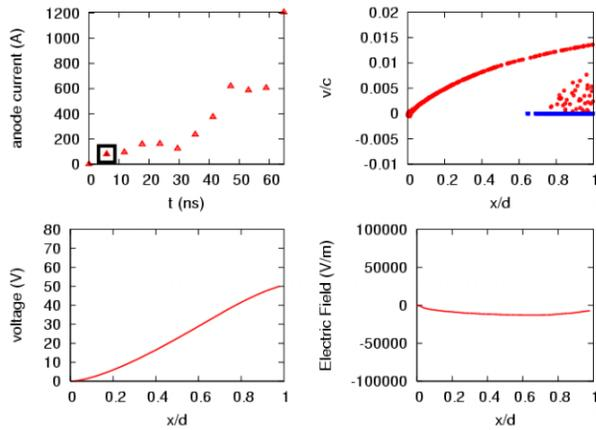
Figure 1: The phase space (upper right), voltage (lower left), and electric field (lower right) at 5ns after the start of electron flow. Ions are shown in blue. For reference, we also show the time history of the anode current (upper left), with the relevant time indicated with a square.
