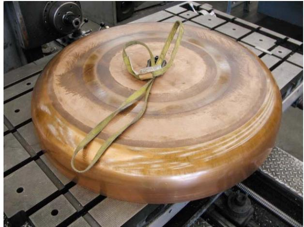
Figure 1: Spun cavity half-shell.
