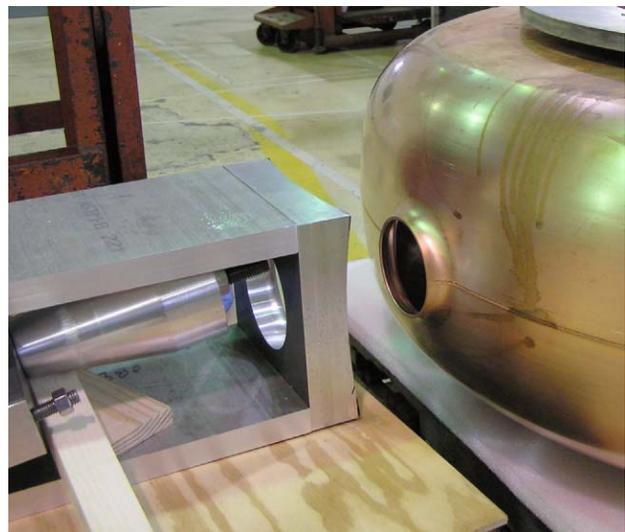
Figure 6. Port pulling after e-beam annealing.
