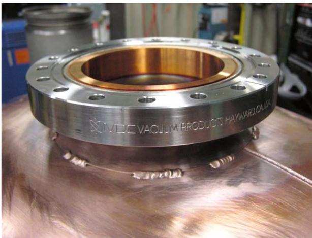
Figure 8. Port repaired by TIG welding.
