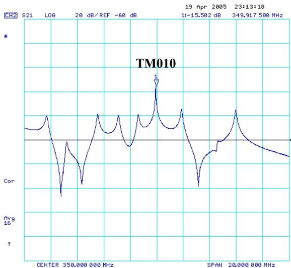
Figure 8: The frequency spectrum near the properly tuned condition
