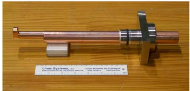
Figure 9b: Post coupler with mounting flange
