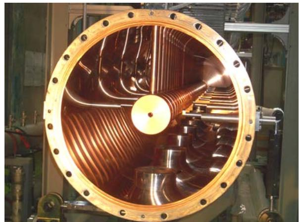
Figure 2: DTL tank 1
