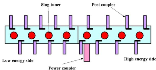
Figure 1: The schematics of the DTL tank1
