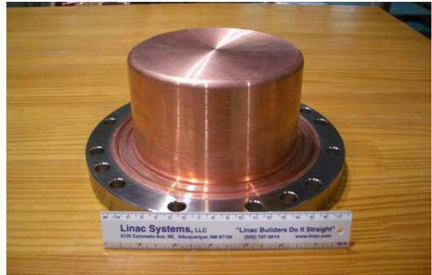
Figure 9a: Slug tuner with STS supporting flange
