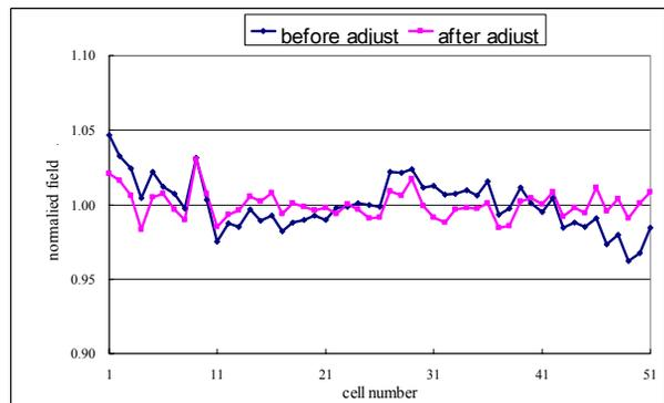
Figure 6: Slug tuner adjustment
