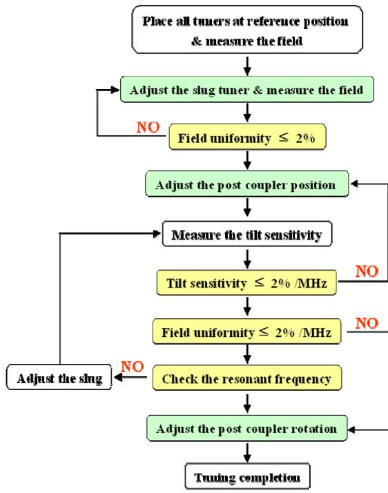
Figure 4: DTL tuning procedure
