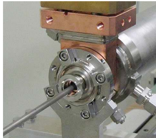
Figure 5: Welding of beamhole plunger.
