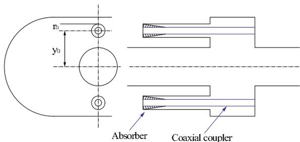
Figure 4: Two coaxial dampers are attached to the squashed cell.
