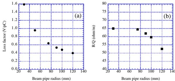
Figure 3: Dependence on the beam pipe radius: (a) the loss factor for  $\sigma_z=3$  mm, and (b) the R/Q value of the crabbing mode.
