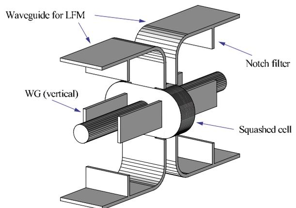
Figure 2: New crab cavity for SuperKEKB (2). Waveguide dampers are used for damping the LFM.
