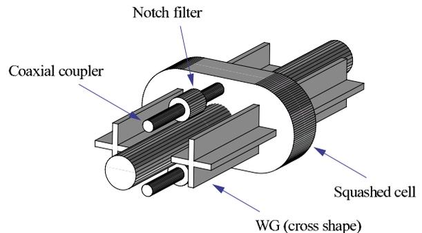
Figure 1: New crab cavity for SuperKEKB (1). Coaxial couplers are used for damping the LFM.
