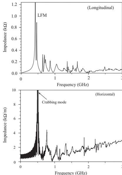
Figure 5: Coupling impedance of the new crab cavity: (upper) longitudinal, and (lower) horizontal.
