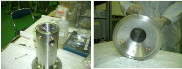
Figure 3: Glass and copper test pieces are attached on the dummy conductor made of stainless steel. A hole was made to inspect the status of the TiN coating inside the conductor, as seen in the left picture.
