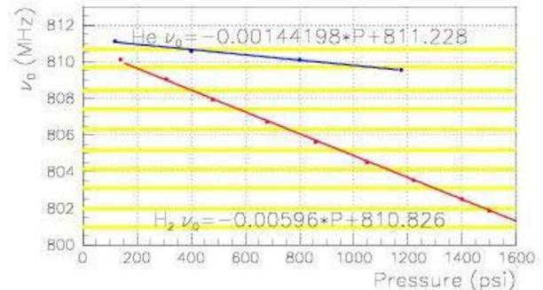
Figure 4: Initial measurements of cavity resonant frequency vs. pressure in the test cell. Horizontal bars indicate resonances in the waveguide. The upper points are  $He$  data and lower points are the  $H_2$  data.
