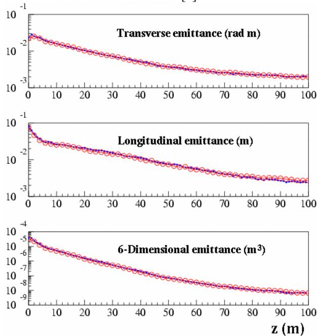
Figure 1: Evolution of emittance over the length of the 100 meter HCC. Results in red are from G4Beamline and blue from ICOOL.
