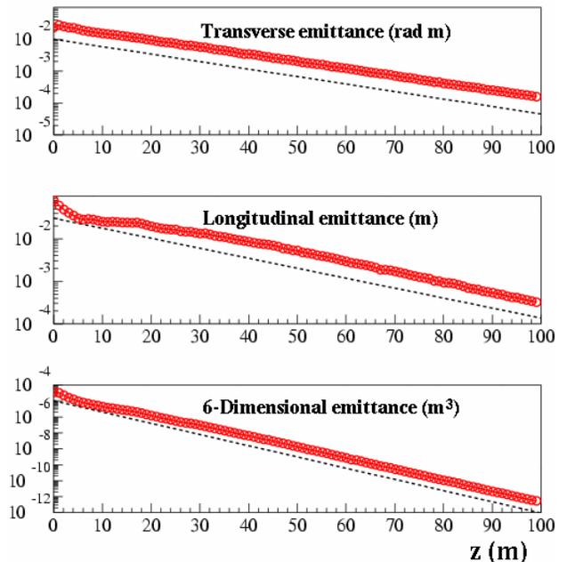
Figure 2: Emittance evolution, as calculated by ICOOL and ECALC9, down the channel with multiple scattering and straggling turned off. The dashed black line shows the predicted slope of the curves, drawn below the simulated data (rather than on top) just to make it easier to see.
