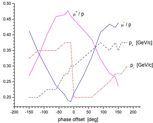
Figure 3: Flux and average momentum of positive and negative particles at the end of the phase rotation channel.
