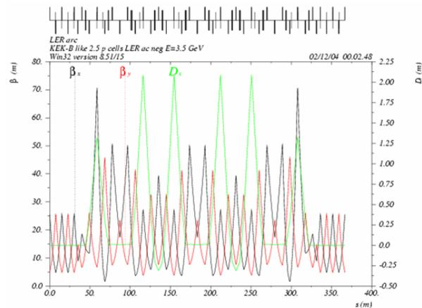
Figure 2: LER lattice with  $2.5 \pi$  phase advance/cell.
