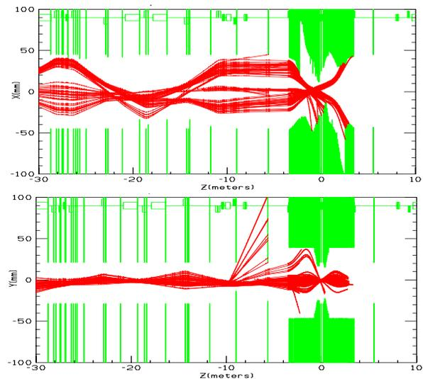
Figure 2: X-Z and Y-Z TOPDRAW plots of Bremsstrahlung particles near the LER IP, located at  $Z = 0$ . Apertures are green, particle tracks are red
