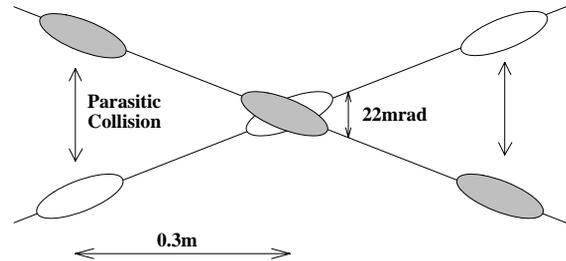
Figure 1: Schematic drawing of the parasitic collision with the finite crossing angle scheme.
