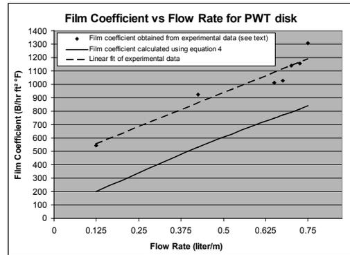
Fig. 4 Disk channel film coefficients, measured vs calculated.
