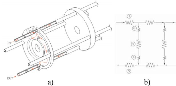
Fig. 1 (a) Cutaway view of disk cooling channel, and (b) elements of a circuit model of flow through two disks.
