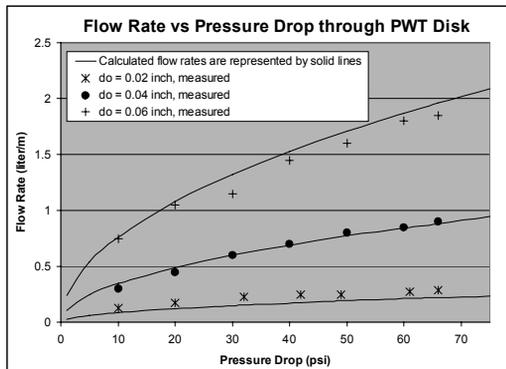
Fig. 3 Disk hydraulic measurements vs calculations.
