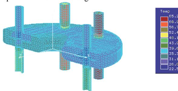
Fig. 6 COSMOS/M 3D finite-element thermal model of a single disk with connecting pipes.
