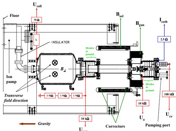
Figure 1: Mechanical drawing of the test bench including an outline of the electrical circuit. and some nomenclature:  $U_a$ , anode voltage;  $U_{ce}$ , control electrode voltage;  $U_{sup}$ , suppressor voltage;  $U_{col}$ , collector voltage;  $I_{cath}$ , cathode current. Plates creating the transverse field are not shown.
