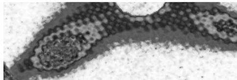
Figure 5: X-Ray CCD image from the injection side of an ECR source plasma showing about half of the plasma region. The extraction aperture is top center. Ionization is occurring in 3 distinct, off-axis, regions [5].
