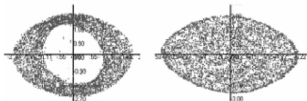
Figure 3: Shapes of  $^{40}\text{Ar}$  beam analyzed to 7+ as calculated with a particle-in-cell model [3]. In the solenoid case (left) effects of 8+ 9+ and 10+ form a ring in x-y space. In the triplet case, but with otherwise identical starting conditions, the beam ring does not form (right).
