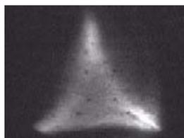
Figure 4: Image of an analyzed  $^{40}\text{Ar}^{7+}$  beam using electrostatic quadrupole focusing under the SCECR.
