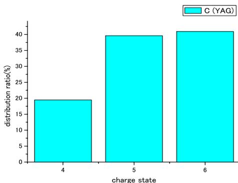
Figure 8: Charge state distribution with YAG-laser.
