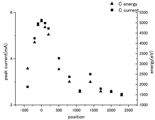
Figure 7: Current change by focus position (C).
