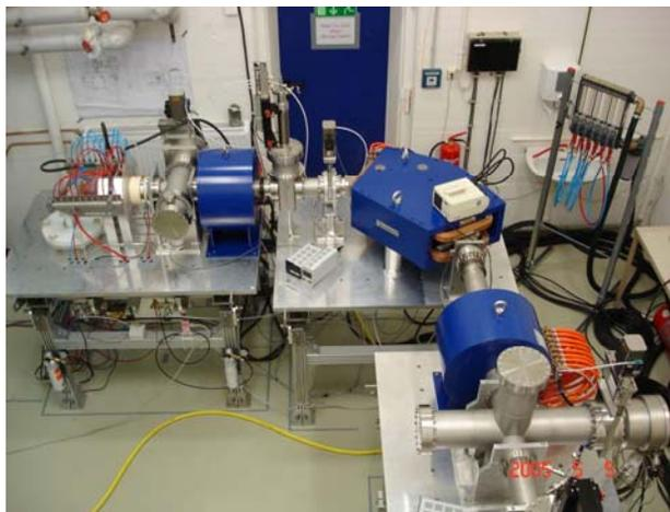
Figure 6: Top view of ECR ion source with LEBT.
