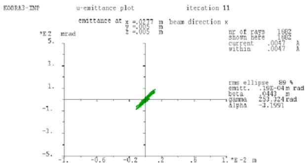
Figure 3: Emittance of simulated deuteron beam.
