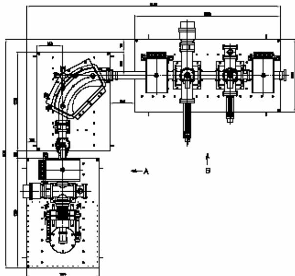
Figure 4: Top view of the ECR Ion Source with LEBT.
