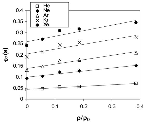
Figure 5: Effusive-flow characteristic time,  $\tau_c$ , as a function of the material density in the target holder.
