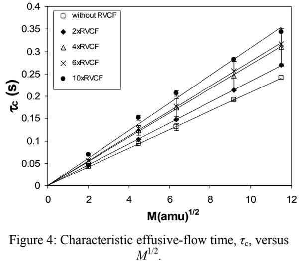
Figure 4: Characteristic effusive-flow time,  $\tau_c$ , versus  $M^{1/2}$ .
