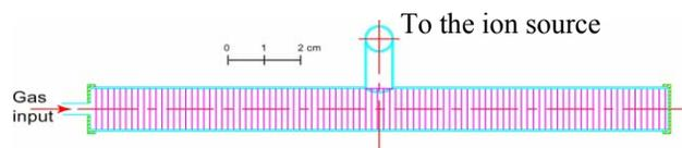
Figure 1: Serial-flow target material reservoir.
